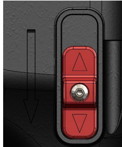
Gear position 2: Low speed, from 30 to 40mm diameter cutters
